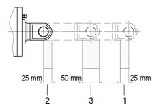
Abb. 7 Permissible setting range of intermediate position
