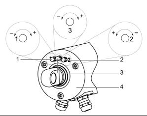
Abb. 6 Cover with setting screw 3 (intermediate position)
