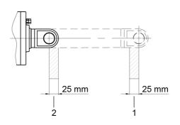
Abb. 4 Permissible stroke reduction
